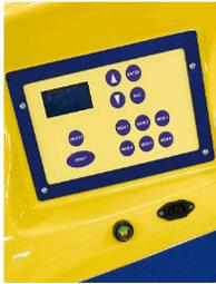
Control panel with **MICROPROCESSOR LOGIC BOARD** <sup>PAT</sup> with the possibility of storing up to 6 different work cycles, each of which with personalized and differentiated parameters.
