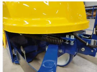
Possibility of **easy spring tension adjustment** thanks to the double hooking system.
