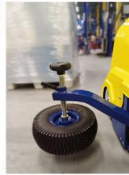
Detection of the dimensions of the load to be wrapped through a touching arm with adjustable height. For better and easier adjustment of the height of the touching wheel, **the robot has been equipped with a lever placed directly on it.**
